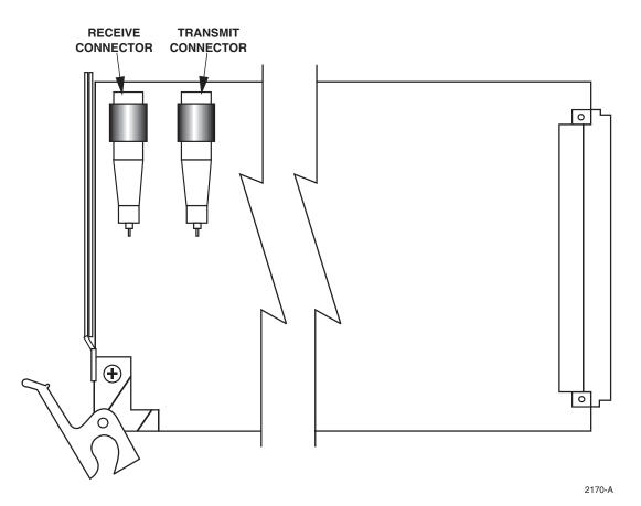
Figure 506-2. ODS2 Transmit and Receive Connector Locations
